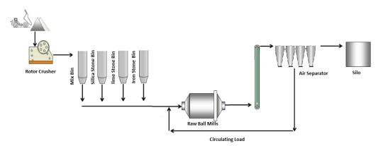
Figure 1. Schematic of ball mill circuit in the Ilam cement plant.
